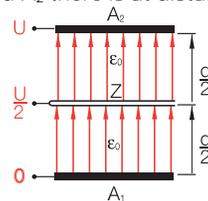
$d/2$  an additional, good conducting, folded „intermediate electrode“  $Z$  with thickness  $D \rightarrow 0$ . An applied voltage between  $A_1$  and  $A_2$  generates an electrical field. This impresses voltage  $U/2$  in electrode  $Z$ . The „intermediate electrode“ thereby assumes the function of an additional capacitor plate. This has the effect of changing the capacitor into two geometrically and electrically series connected capacitors.
