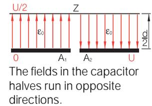
The fields in the capacitor halves run in opposite directions.
